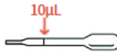
Use the capillary transfer tube collect 10ul blood samples, squeeze the tube into the test strip blood slot
