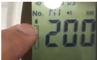
Top left corner of the screen will blink, meter is waiting for add blood sample
