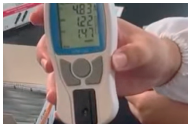
After adding the sample in 120 seconds, the screen will show the result
